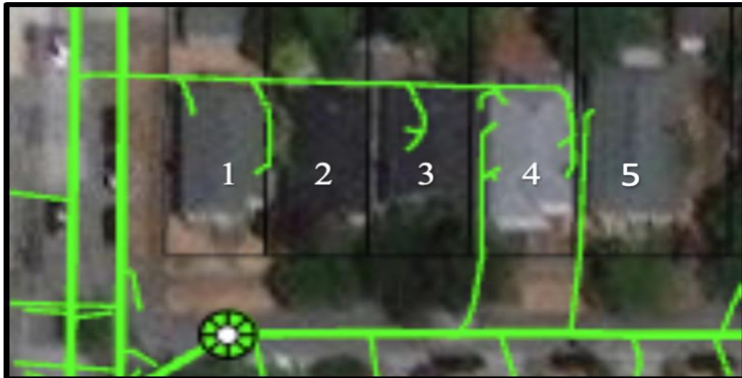
Figure 11: Note structure 4 is connected to 2 mainlines and has 3 other structures on one lateral. Additionally, the need for good accuracy of field locations is illustrated by the closeness of two laterals at the property line between 4 and 5.
