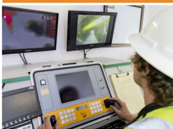
A technician with PSE service partner Hydromax USA places a robotic camera down a sewer to inspect for a natural gas pipeline, visible on the monitor below.
