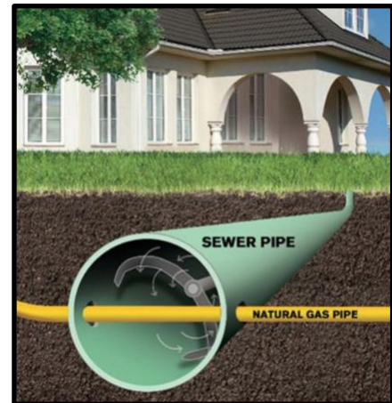
Figure 1: House sewer lateral with cross bore
