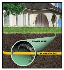
Figure 1: Graphic of sewer cleaning risk of a gas cross bore in sewer
