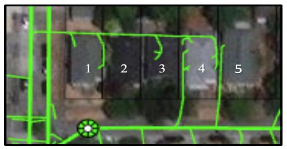
Figure 11: Note structure 4 is connected to 2 mainlines and has 3 additional structures on one lateral. Additionally, the need for good goe-location accuracy of field locations is illustrated by the closeness of two laterals at the property line between 4 and 5.
