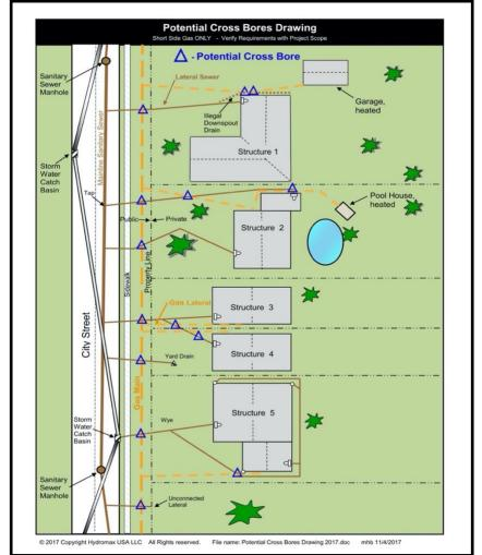
Figure 6: Potential cross bore intersections, shown as  $\triangle$ , of gas and sanitary sewers. Storm sewer intersections NOT shown. Short side gas ONLY, laterals on same side of mainline.
