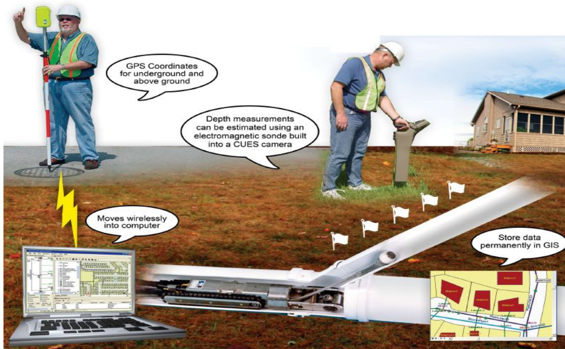
Figure 6: The Technologies Used: GIS Software, Wireless GPS, Digital Video, Sonde and Robotic transporter.
