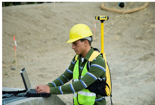
Figure 12 : GPS Backpack kit for Sub-centimeter survey grade data collection (alternative)
